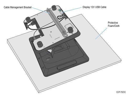
13. Connect the USB cable to the connector at back of the base.
