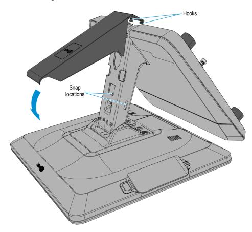
16. Mount the Neck Cover. Hook the Cover to the rear side of the Neck then rotate downward and press the Neck Cover until it latches on to the Neck.
