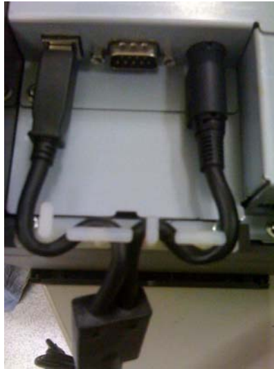
Current Cable Retention Method
