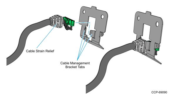
2. Connect the USB Cable to the Customer Display. Note the cable routing (Cable Management Bracket removed for clarity).
