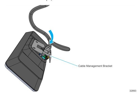
4. Pivot the Cable Management Bracket until it snaps into position.
