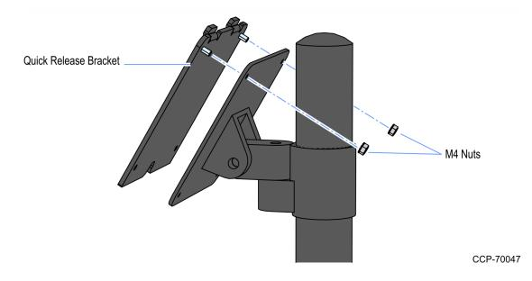
2. Mount the Display on the Mounting Plate Studs of the Quick Release Bracket at a slight angle as shown.
