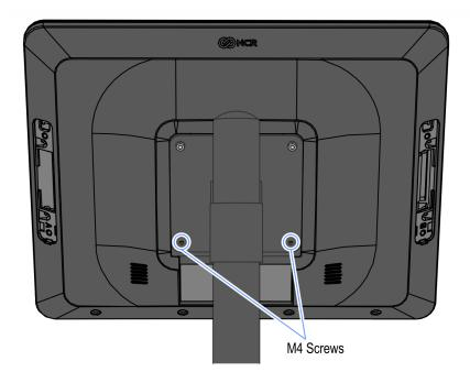
3. Rotate the Display flush onto the Bracket and secure it with two (2) M4 screws.
