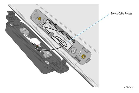
3. Insert the hook of the MSR into the rectangular hole on the Display Head and press the other end to mount the MSR. Make sure the cable does not get pinched.
