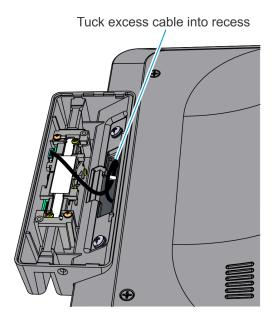
6. Hook the MSR Rear Cabinet into the Front Cabinet and pivot to close. Secure with a screw.
