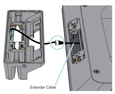
4. Install the MSR Front Cabinet on the Display Head (2 screws).
