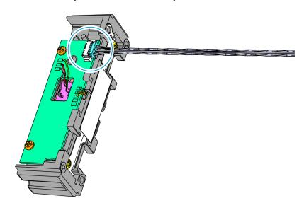
2. Install the JIS MSR on the MSR Front Cabinet (2 screws).
