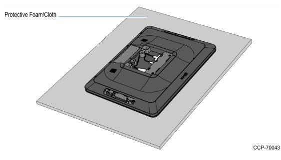
2. Insert the Mounting Plate Studs (2) into the openings on the back of the display at a slight angle as shown.
