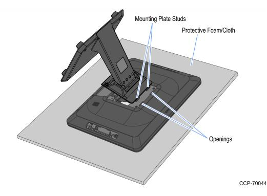
3. Rotate the stand flush into the back of the display and secure it with screws (2). Use the appropriate screws for the display.
