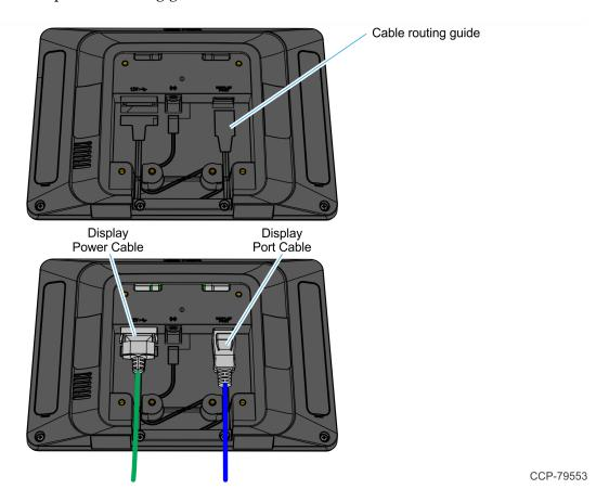
2. Route the Cables through the opening as shown, then insert the Hinge Plate tabs into the slots in the rear of the Display and slowly rotate the Display onto the Plate.
