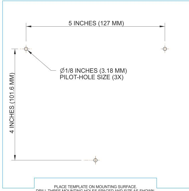
DRILL THREE MOUNTING HOLES SPACED AND SIZE AS SHOWN.
