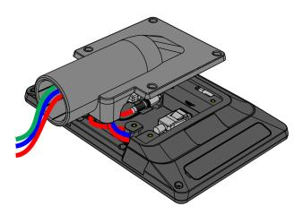
3. Install the Bracket on the back of the Display (4 screws).
