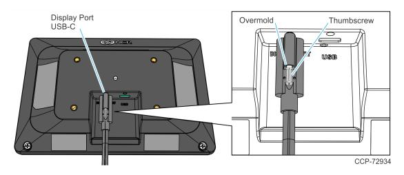
2. Route the cable through the Display Mount Bracket and install the bracket on the back of the display (4 screws).
