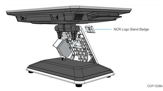
d. Route the cable through the stand. Secure the Bracket and Display assembly from the inside of the stand (2 screws).
