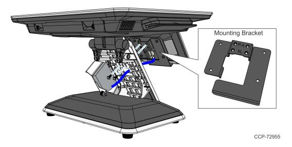
e. Route the cable up the stand and connect the cable to the host terminal. Close and secure the Base Cable Cover with the thumbscrew.
