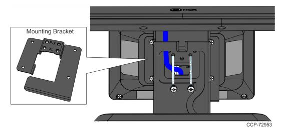
c. Connect the cable to the host terminal.
