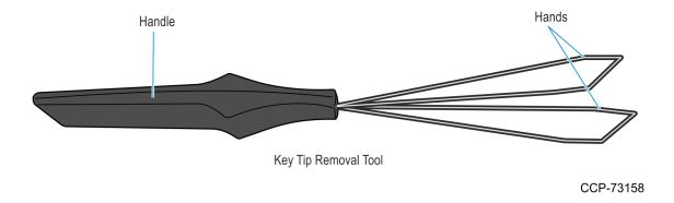
Insert the hands of the removal tool under each side of the Key Tip and carefully pull the tool upward until the Key Tip pops off its retainer clips.
