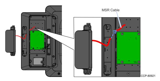
5. Insert the hook of the MSR into the rectangular hole on the Enhanced Keypad and press the other end to mount the MSR. Make sure the cable does not get pinched.
