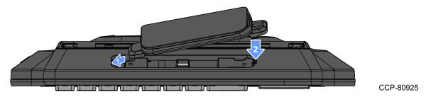
6. Secure the MSR to the Enhanced Keypad with a screw.
