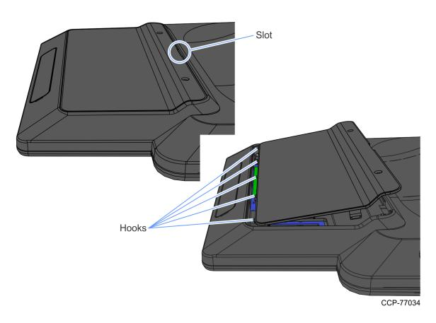
3. Use a screw driver to unlatch the recessed side of the Filler Plate and then slightly pull the Filler Plate to unhook from the Enhanced Keypad.
