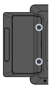
2. Insert a flat screw driver in the slot to unsnap the Rear Cover, then unhook the Rear Cover from the Keypad housing.
