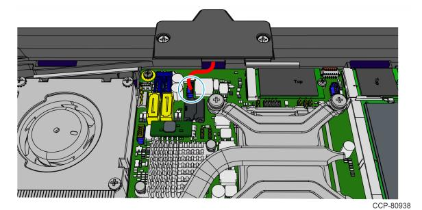
6. Install the Camera on the display housing (2 screws).
