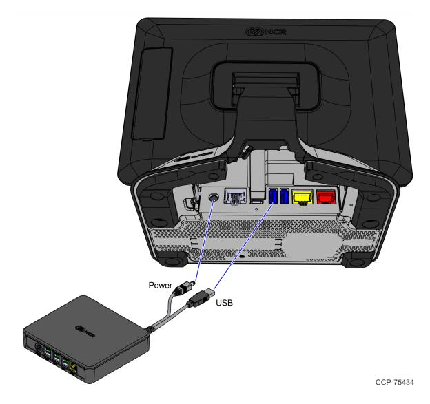
2. Connect the Power Supply Cable to the Expansion Box.
