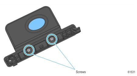
Confidential and proprietary information of NCR Voyix. Use and disclose solely pursuant to company instructions. b. Rotate the UV Light module until it is detached.
