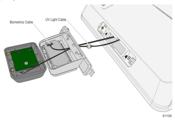
Confidential and proprietary information of NCR Voyix. Use and disclose solely pursuant to company instructions. 4. Snap the UV Light into the bracket. Ensure the snaps are fully engaged.
