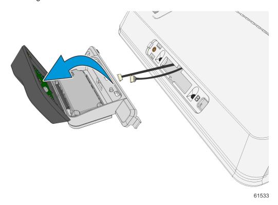
3. Route and connect the Biometrics and UV Light cables to the corresponding connectors through the opening in the bracket.
