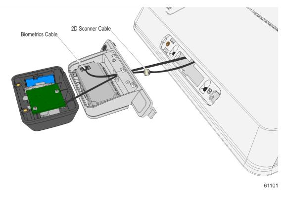
4. Snap the 2D scanner into the bracket. Ensure the snaps are fully engaged.
