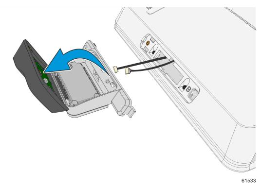
3. Route and connect the Biometrics and 2D Scanner cables to the corresponding connectors through the opening in the bracket.
