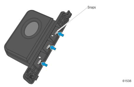
Confidential and proprietary information of NCR Voyix. Use and disclose solely pursuant to company instructions. b. Rotate the Bottom Blank until it gets detached.
