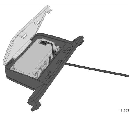
Confidential and proprietary information of NCR Voyix. Use and disclose solely pursuant to company instructions. 4. Snap the bottom blank into the bracket. Ensure the snaps are fully engaged.
