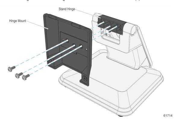
5. Install the Hinge Mount over the Expansion Board assembly.
