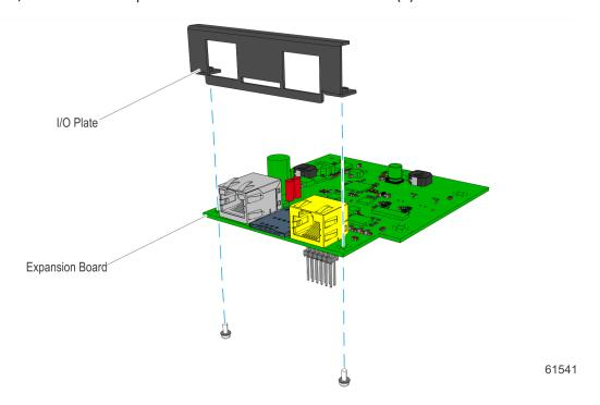
3. Install the Expansion Board assembly into the funnel and secure to standoffs with screws (4).
