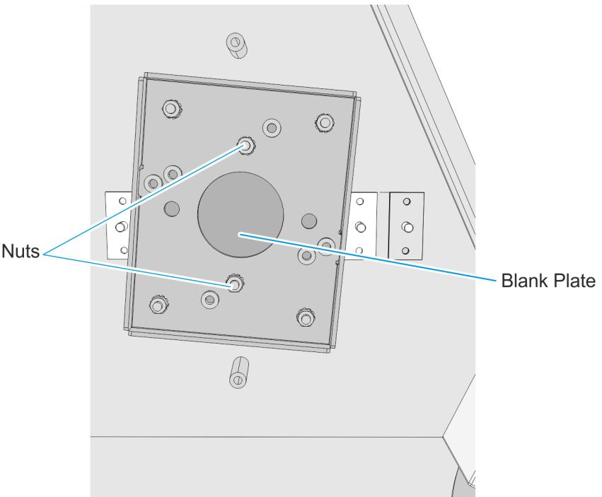
3. Insert the mounting studs of the angular arm through the mounting holes on the cabinet and secure the arm with nuts (4).
