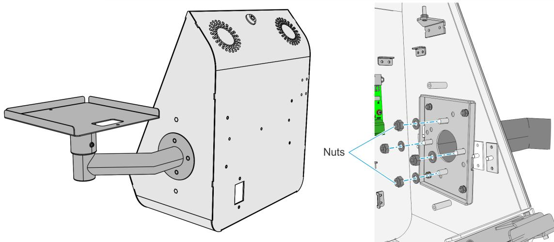
4. Re-install the power supply bracket and the power supply.
