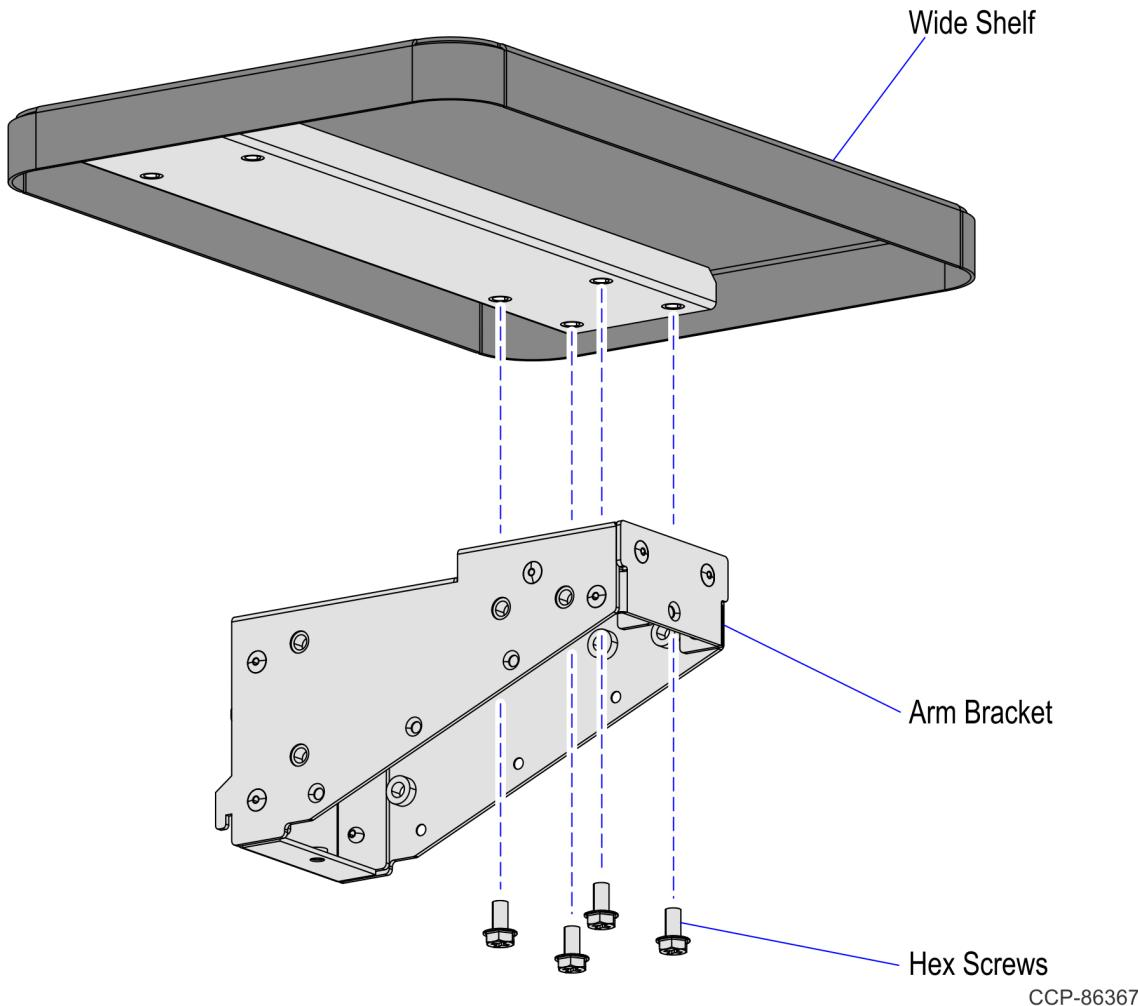
b. Attach and tightly secure the Front Support Bracket (Right-Hand) to the Shelf and Arm bracket using four (4) hex screws, as shown in the image below.
