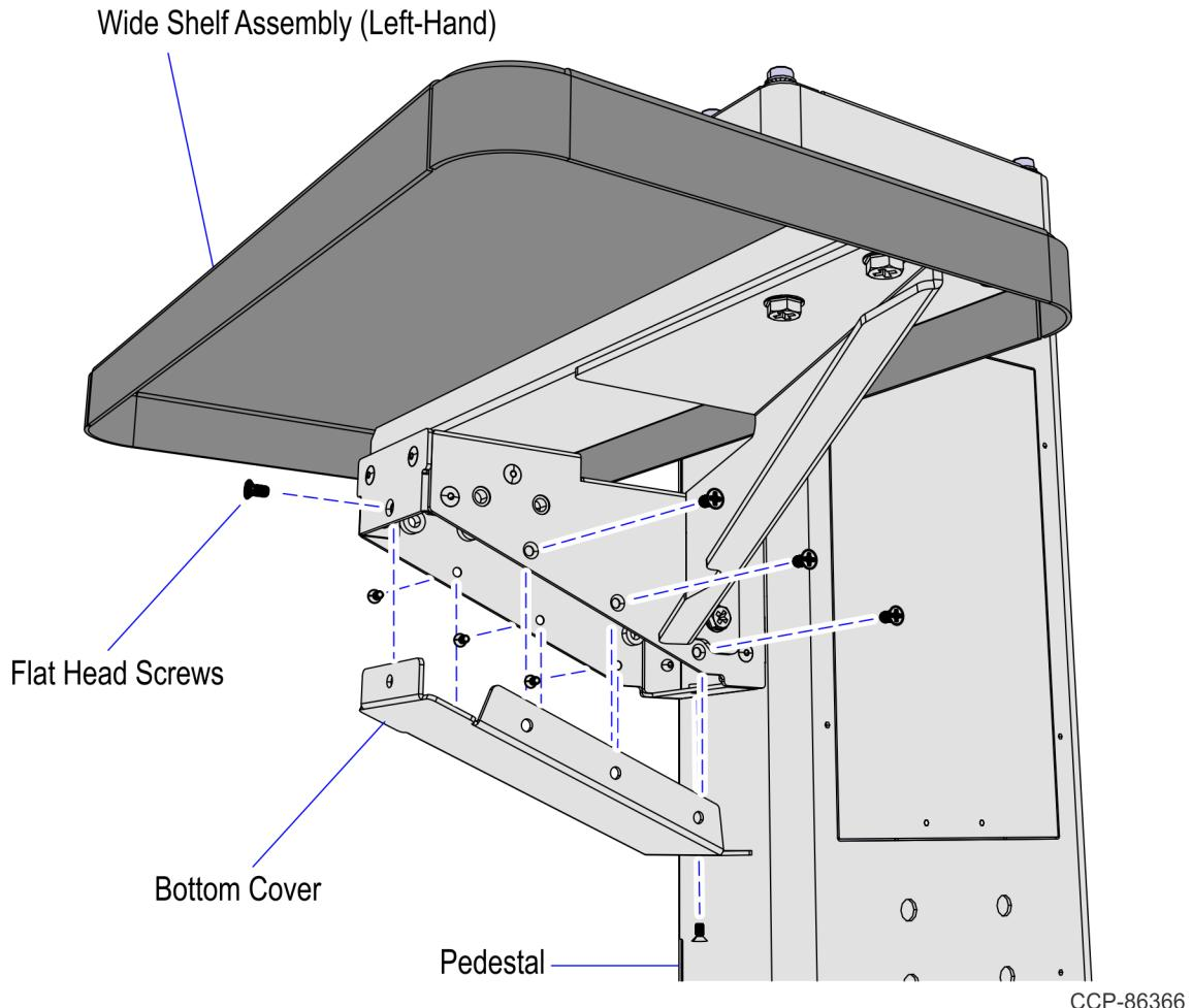
2. Remove two (2) hex screws to detach the Wide Shelf assembly from the Pedestal.
