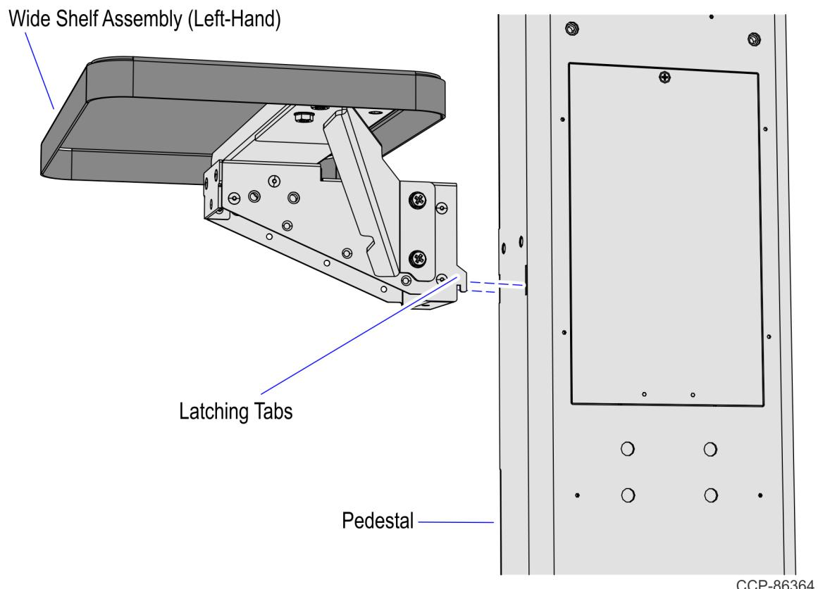
3. Tightly secure the Wide Shelf assembly to the Pedestal using two (2) hex screws.
