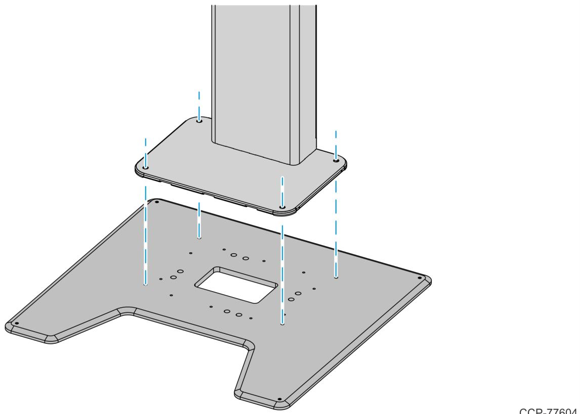
3. Secure the pedestal with four M8x20mm screws and four washers.
