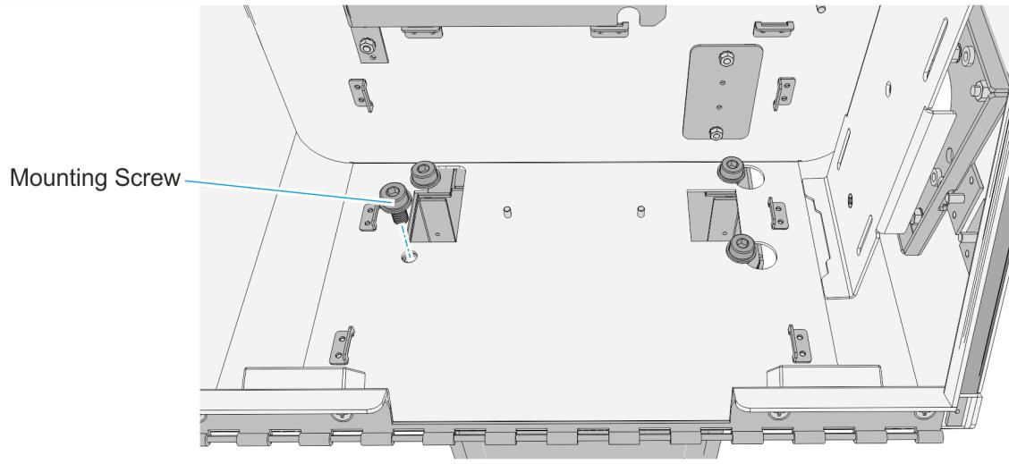
10. Cover the following mounting holes using the SS90 Hole Cover Label if there are no side shelves, front shelf, or bagger to be installed to the pedestal.
