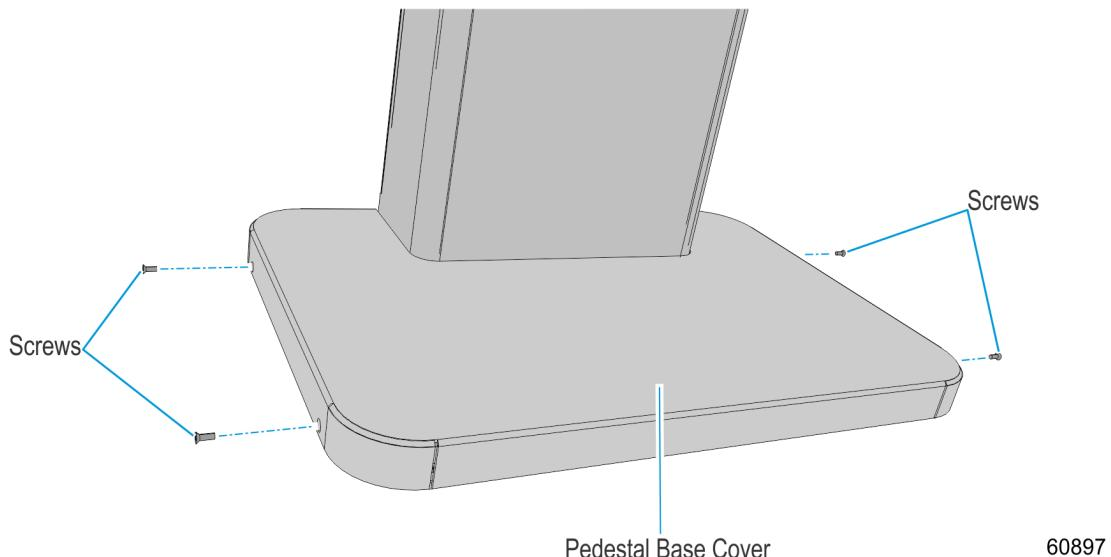
3. Mark the anchor holes (4) in the pedestal base on the floor. Remove the pedestal.
