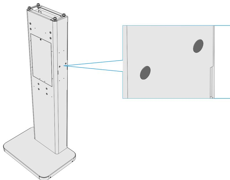
b. **Front mounting holes** - cover holes if kit 7709-K434 (Bagger with Shelf) will not be installed. There are four (4) mounting holes each for the bagger and shelf.
