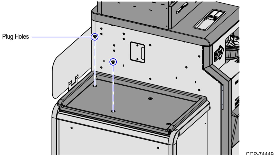
2. Align the Japan Bag Rack with the two screw holes on the Scale Tray.
