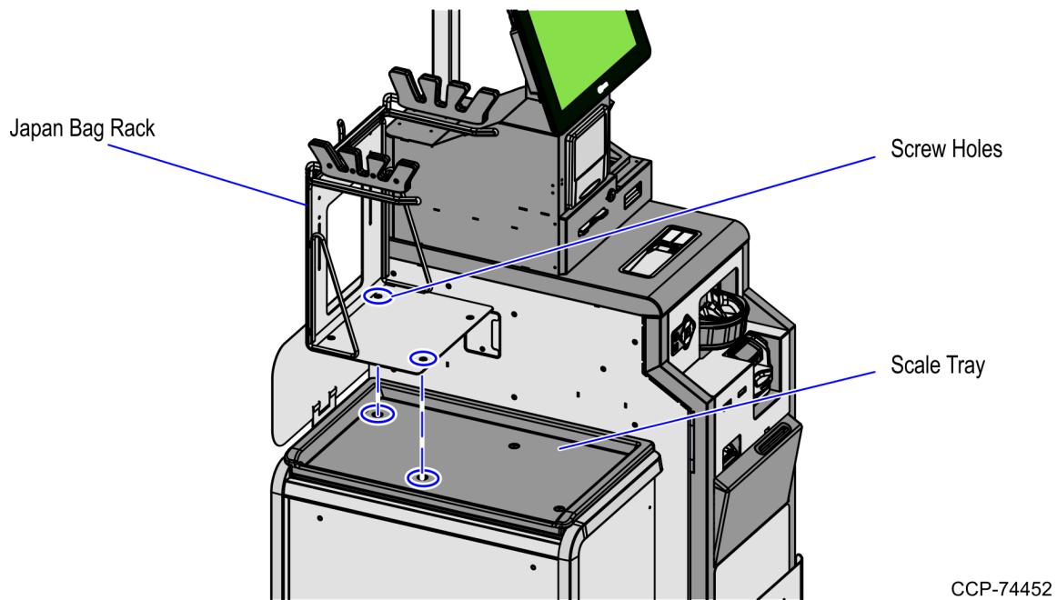
3. Secure the Japan Bag Rack to the Scale Tray using two M6 Flat-head screws.
