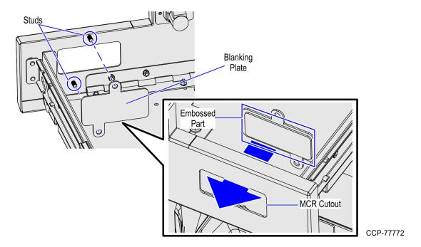
3. Secure the Blanking Plate to the Upper Cabinet Door using two (2) nuts, as shown in the image below.
