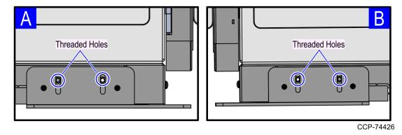
3. Fasten each Stabilizer Bracket using two M6 Bolts with wedge lock washers as shown below.
