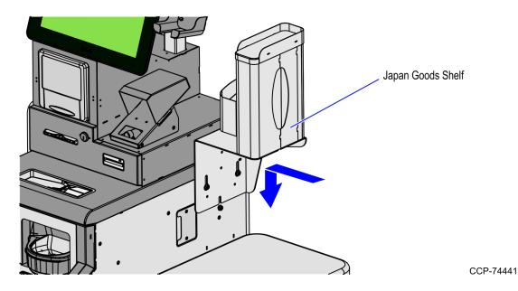
4. Tighten all three screws to secure the shelf to the unit.
