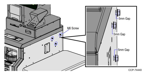
3. Align the Japan Goods Shelf slots with the corresponding M6 Screws and then slide the shelf down onto screws.
