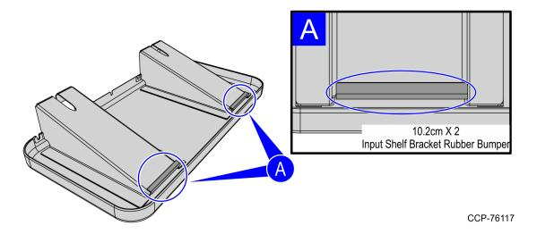
2. On the slotted edge of each Input Shelf Bracket, insert two (2) 6.8 cm rubber bumpers on each edge of a slot, as shown in the image below.
