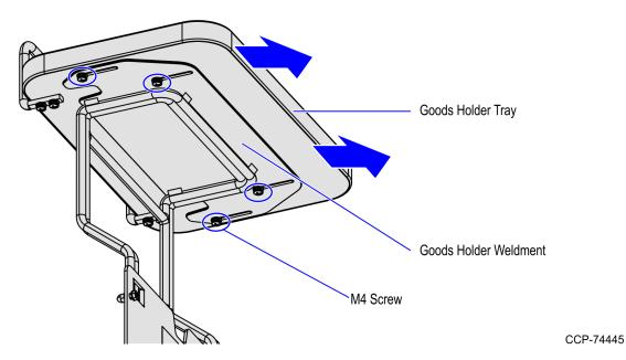
**Note:** The default Goods Holder Tray configuration should be fully extended forward as shown in the image below.
