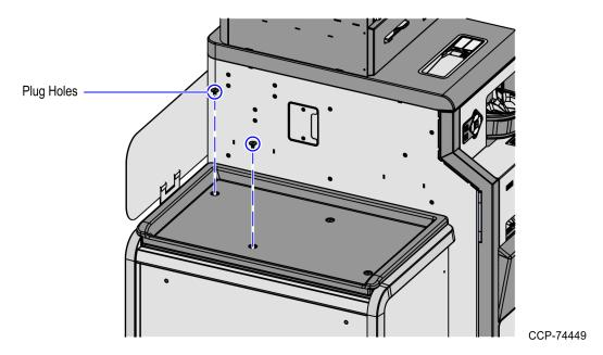
3. Align the Japan Bag Rack assembly with the two screw holes on the Scale Tray.
