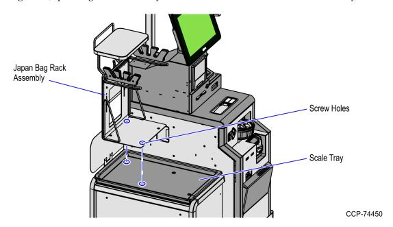
4. Secure the Japan Bag Rack to the Scale Tray using two M6 Flat-head screws.
