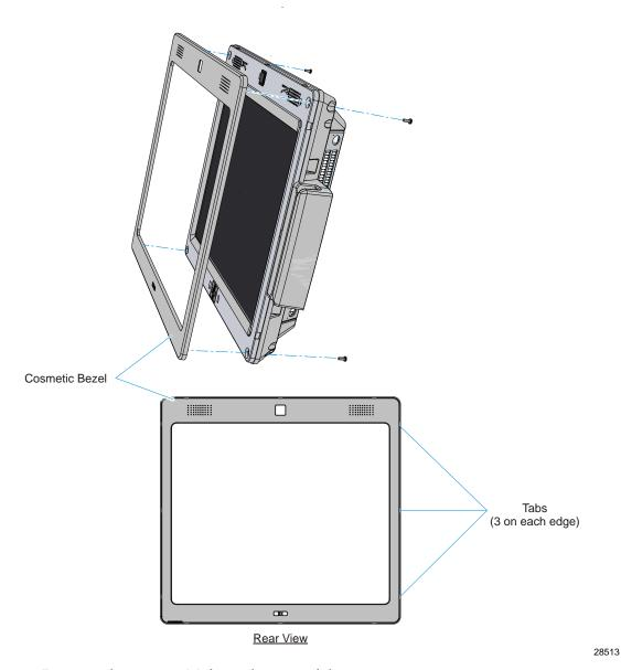
1. Remove the screws (4) from the rear of the unit.
