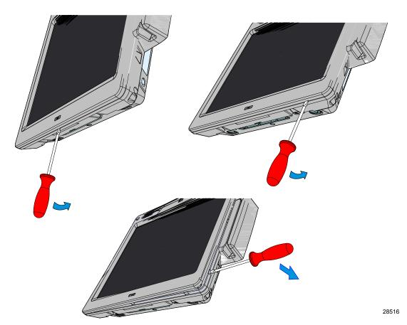
After releasing the center latch repeat the procedure for the two latches holding the lower corner. By then you can get your fingers under the bezel and release the remainder of the latches by hand.
