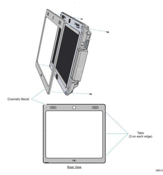
1. Remove the screws (4) from the rear of the unit that secure the bezel.
