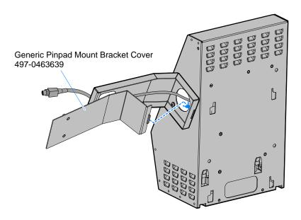
9. Secure the Generic Pinpad Mount Bracket Cover with screws (2), enclosing the cable.
