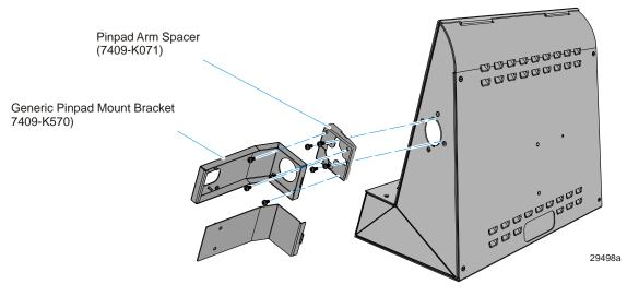
7. Route the device cable through the openings in the bracket and into the Fixed Angle Mount.
