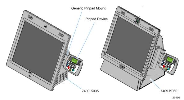
The mount is used in conjunction with device specific mounting bracket kits to install the various pinpads.
