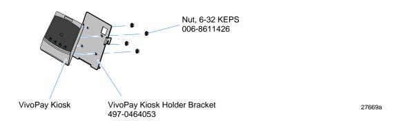
4. Secure the VivoPay Kiosk/Holder Bracket Assembly to the VivoPay Kiosk Mount Bracket (two hooks and a screw from the bottom).
