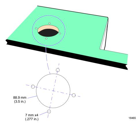
2. Place the Swivel Mount Bracket into the hole.
