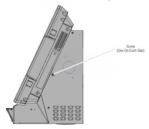
b. Tilt the display as shown and rest the display on the Display Support.
