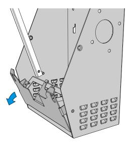
5. Hook the bottom of the new Scanner Faceplate onto the bottom edge of the opening on the Fixed Angle Mount and then secure the assembly with screws (2).
