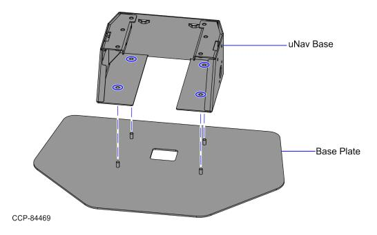
2. Secure the uNav Base to the Base Plate using four (4) M6 nuts.
