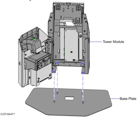
3. Secure the Tower Module to the Base Plate using four (4) M6 nuts.
