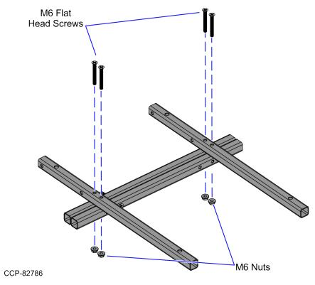
4. Insert the support bar assembly into the Gusset and secure using four (4) M6 flat head screws and nuts.
