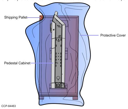
5. Position the Pedestal Cabinet so that its rear is on the protective cover.
