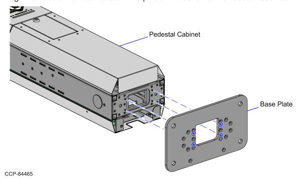
7. Secure the Base Plate to the bottom of the Pedestal Cabinet using 16 M6 screws.
