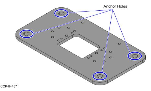
3. Install the anchors in the marked locations based on the manufacturer's instructions.
