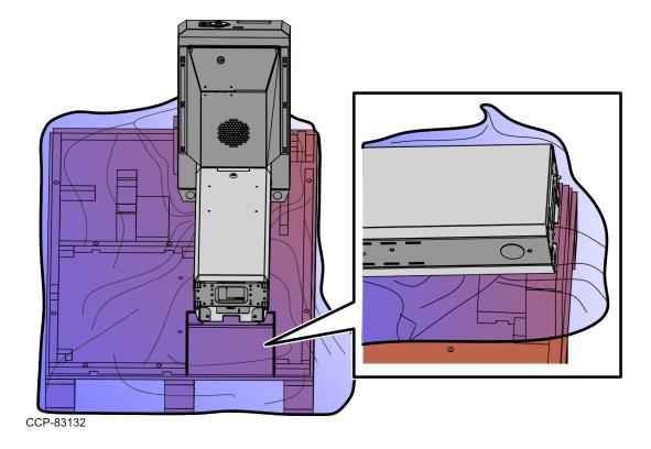
3. Align the holes of the Base Plate with the pins on the bottom of the Pedestal Cabinet.
