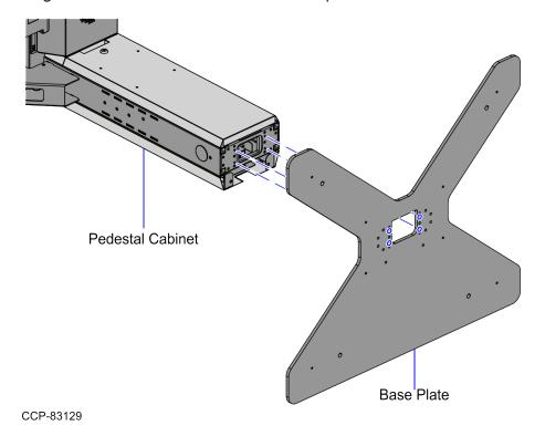
4. Secure the Base Plate to the bottom of the Pedestal Cabinet using 16 M6 screws.
