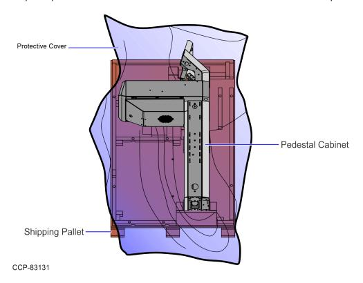
2. Position the Pedestal Cabinet so that its rear is on the protective cover.
