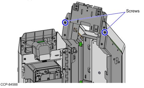
3. Detach the Rear Cosmetic Cover from the Tower Frame by disengaging two (2) hooks from the Tower Frame tabs.
