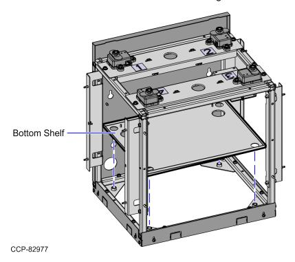
6. Attach the Bagwell Stabilizer to the Bagwell Frame using four (4) screws, as shown in the image below.
