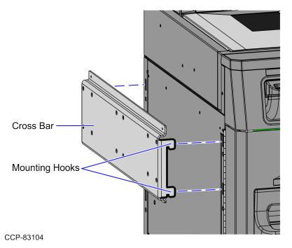
3. Using two (2) M3 screws, secure the Cross Bar to the Core Cabinet.
