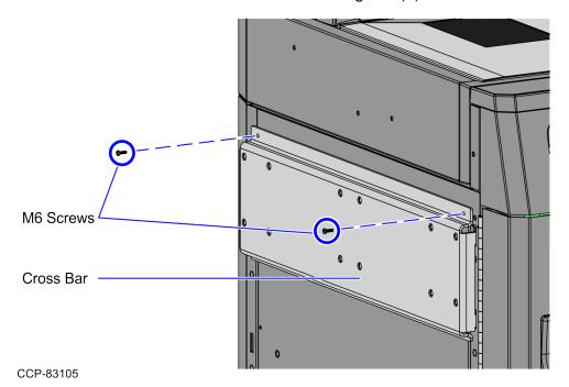
4. Attach the Input Shelf Top assembly to the Cross Bar using four (4) M6 screws, as
