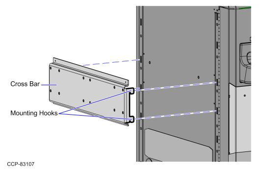
3. Secure the Cross Bar to the Core Cabinet using two (2) M3 screws.
