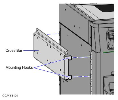
3. Secure the Cross Bar to the Core Cabinet using two (2) M3 screws.
