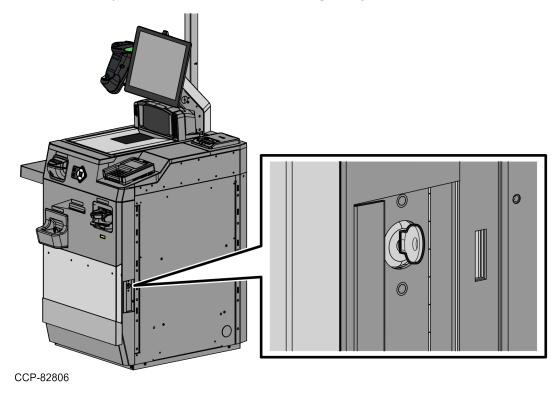
Confidential and proprietary information of NCR. Unauthorized use, reproduction and/or distribution is strictly prohibited. 2. Hold and press the self-locking mechanism at the back of the Coupon Bin Blank to release it from the Coupon Chute.
