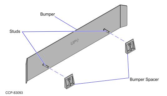
3. Insert the Bumper Studs with Spacers into the corresponding holes on the Cosmetic Door, as shown in the image below.
