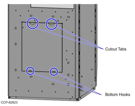
2. Slowly pull the back panel forward to disengage the bottom hooks from the Core Cabinet, as shown in the image below.
