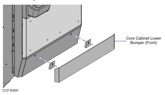
4. Secure the Bumper assembly to the Cosmetic Door using two (2) nuts, as shown in the image below.
