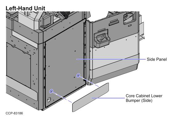
5. From inside the Core (Cabinet), secure the Bumper to the Side Panel using two (2) nuts.
