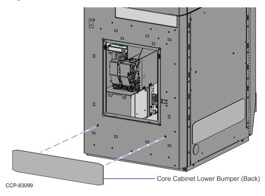
3. Secure the Bumper to the Core (Cabinet) using two (2) nuts.
