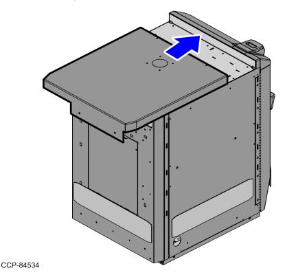
3. Secure the CTM Top Plate Cover at the rear of the Top Plate using two (2) screws, as shown in the image below.
