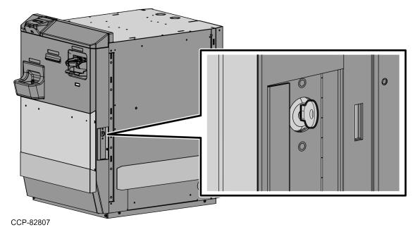
5. Secure the CTM Top Plate Cover from inside the Core (Cabinet) and under the Top Plate using one (1) nut, as shown in the image below.
