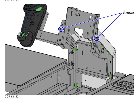
10. Slide the Terminal Display down the Display Support and then secure it using a thumb screw, as shown in the image below.
