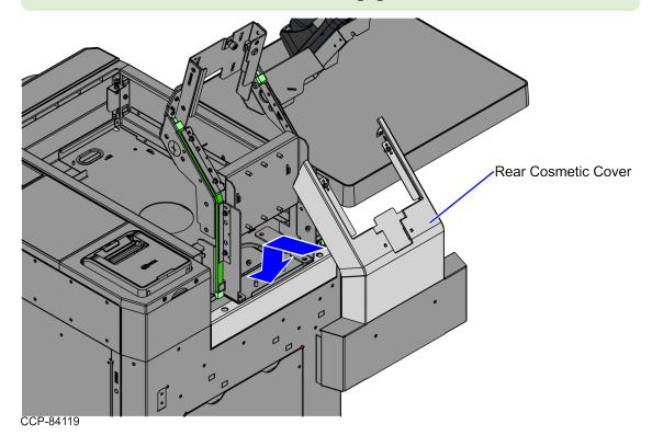
9. Secure the Lower Rear Cosmetic Cover to the Tower Frame with two (2) screws.
