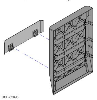
3. Secure the Bumper assembly to the Bagwell Front Panel using two (2) nuts.
