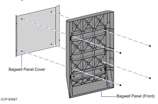
2. Secure the Cover to the Bagwell Front Panel using four (4) nuts.
