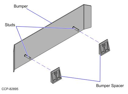
2. Insert the Bumper Studs with Spacers into the corresponding holes on the Bagwell Front Panel, as shown in the image below.
