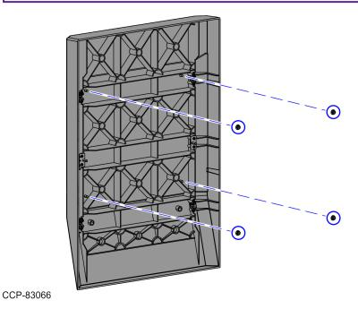
2. Detach the Cover from the Bagwell Front Panel, as shown in the image below.
