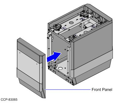
2. Secure the Panel to the Bagwell Frame using two (2) wing nuts from inside the Bagwell, as shown in the image below.
