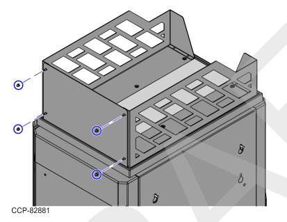
2. Remove four (4) screws to detach each Fence from the Scale Tray.
