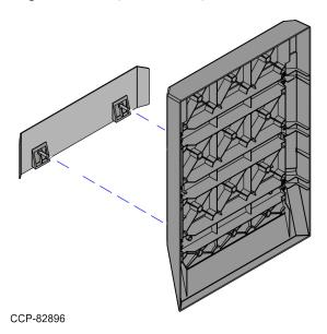
c. Secure the Bumper assembly to the Bagwell Panel (Front/Back) using two (2)
