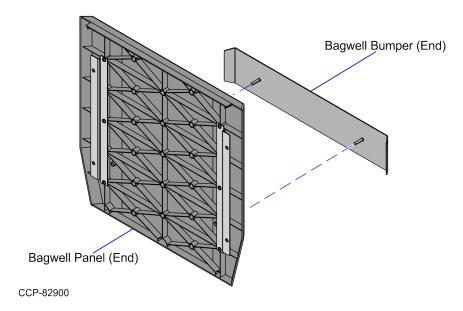
b. Secure the Bumper to the Bagwell End Panel using two (2) nuts.
