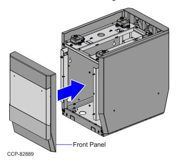
2. Secure the Front Panel from inside the Bagwell Frame using two (2) wing nuts, as shown in the image below.
