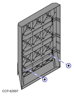
6. Install the Front Panel to the Bagwell Frame. For more information, refer to <u>Installing</u> the Bagwell Front Panel.
