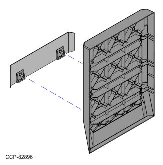
5. Secure the Bumper assembly to the Bagwell Front Panel using two (2) nuts.
