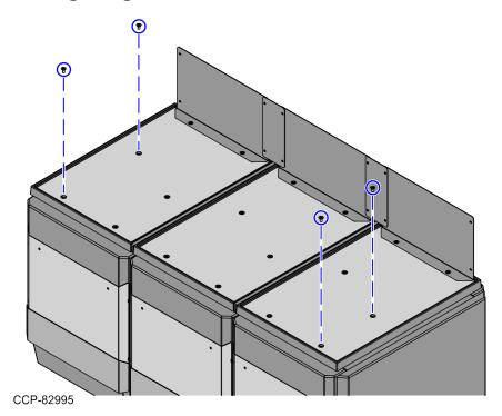
2. Align the screw slots of each Fence with the corresponding mounting holes on the Scale Tray.
