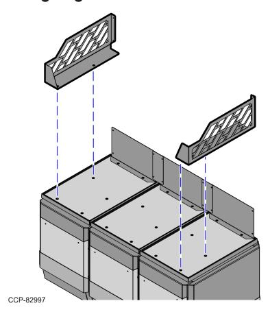
3. Secure each Fence on the Scale Tray using four (4) screws.
