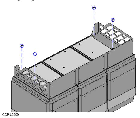
4. Secure the Fence to the Backsplash using four (4) nuts, as shown in the image below.
