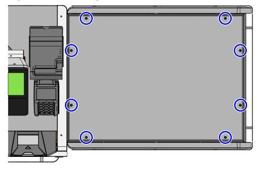
3. Align the screw slots of the Scale Tray Fence to the corresponding mounting holes on the Scale Tray.
